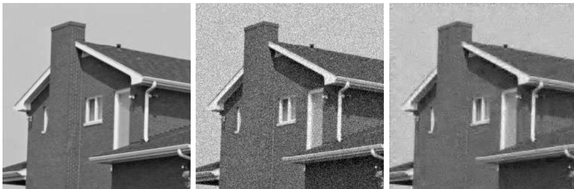
Figure 6: Result of the threshold operation with the minimizer of GCV(\delta) , based on 1000 pixels. On the left hand we have the original image, in the middle the noisy image ( SNR = 10.0\text{dB} ), on the right the result ( SNR = 15.5\text{dB} ).
